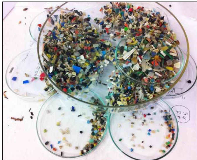
Figure 2: Marine plastic fragments sorted by size in the lab (photo: Paula Sobral)
